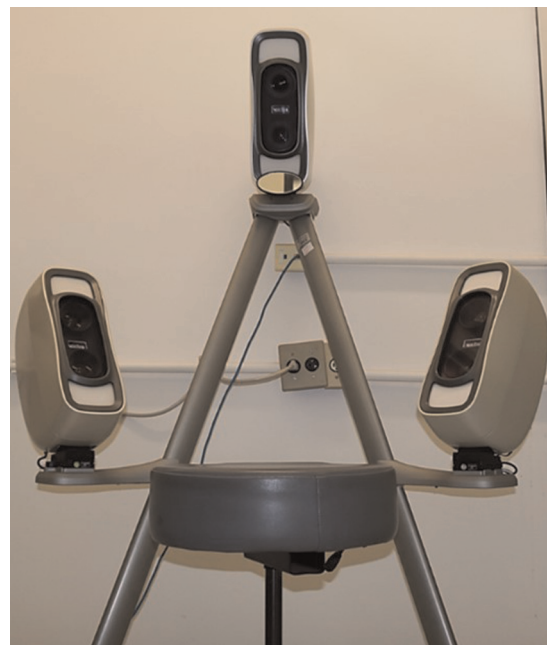
Figure 1: Digital stereophotogrammetry device used to obtain the 2D and 3D images (VECTRA M3®, Canfield Scientific Inc., Fairfield, New Jersey, USA)
